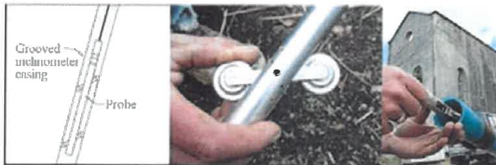
Figure 9 - Portable Inclinometer Probe (Read & Stacey, 2009)
