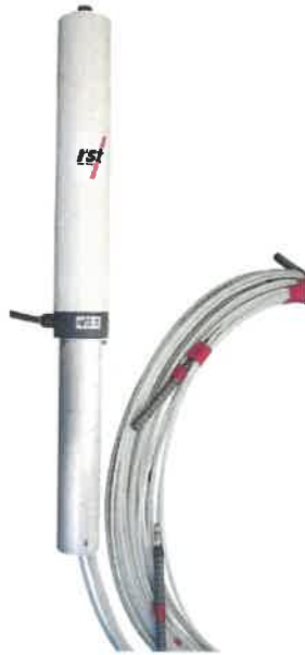
Figure 11 - Borehole Extensometer (RST Instruments, 2023)
